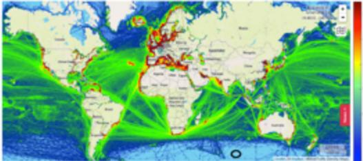
Fig. 1. 2012 worldwide maritime traffic density map. The density is evaluated as the number of ships per 1° x 1° grid cell per day (from [www.marinetraffic.com](http://www.marinetraffic.com)). The black circle indicates the region selected in the third (ocean floor) scenario. Cyan background indicates regions with no sea traffic.
